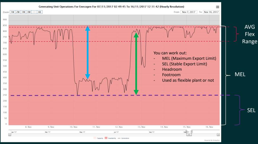
Headroom: Difference between running level and max capacity, also UPWARD MARGIN
